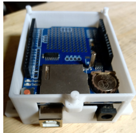
Figure 13. Bottom printed box with ARDUINO UNO
